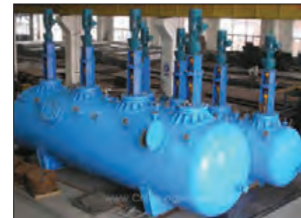
Beneficiation equipment: autoclave for hydrometallurgy.
